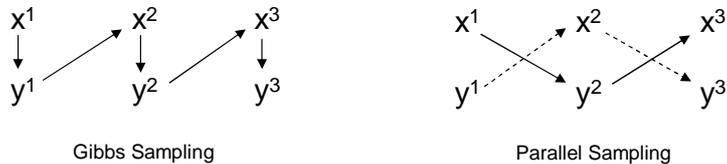
Figure 2: Sampling two variables in parallel, conditioned on the opposing value in the previous time step, produces two independent chains and incorrect results [34].
